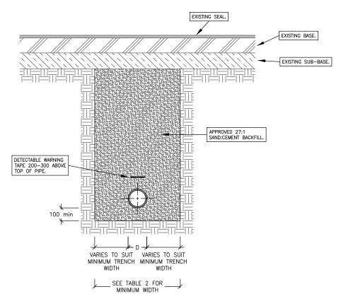
CASE 1: PIPES UNDER EXISTING TRAFFICABLE SURFACE OR WITH COVER LESS THAN 800
