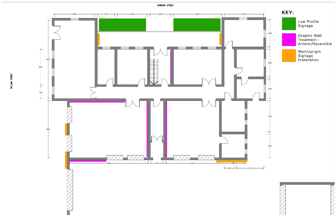
Figure 48 Location for various on-site interpretation devices depending on decided usage. Note: It is not recommended to use all of these places concurrently, it shows opportunities to suit future requirements.
