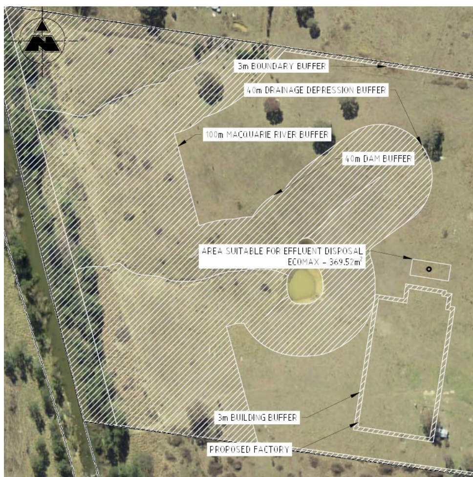
Figure 5 – Proposed effluent disposal area for non-plant related wastes. Source: Calare Civil Consulting Engineers – Effluent Disposal Investigation – 1673 Freemantle Road, Watton NSW 2795 dated 30 August 2021.
