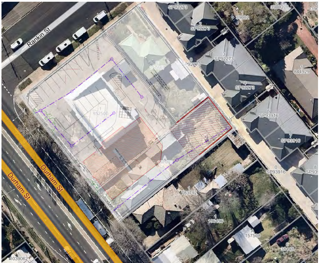
Figure 11 – Relationship of Earthworks and Retaining Walls to Neighbouring Residential Properties – Fill and Retaining Walls (Shown Dark Red) with a Maximum Height of 1 metre Proposed at Eastern End of Site (Lot A DP 197473, 105 Durham Street)
