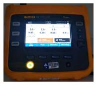
R22 inverter 8kW Cooling Running Amps = **9.87 A**
