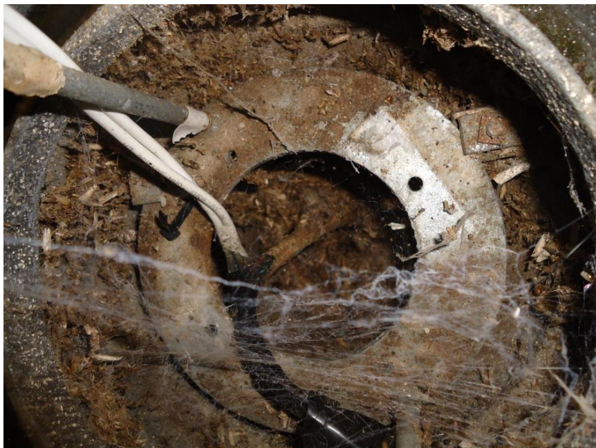
Photo 2: Insect build up in the Lamp Base
