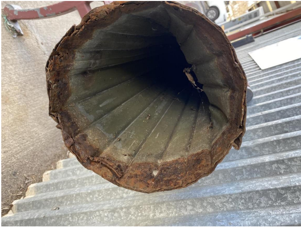
Photo 34: Corroded base of rolled galvanised post from Machattie Park and Kings Parade Lamp Standard
