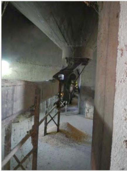
Figure 242 Pipes to carry the grain from the concrete silos (© Kasiannan)
