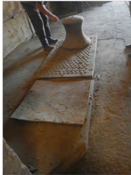
Figure 206 A capstan, that helped move rail carriages. (© Kasiannan, 2016)
