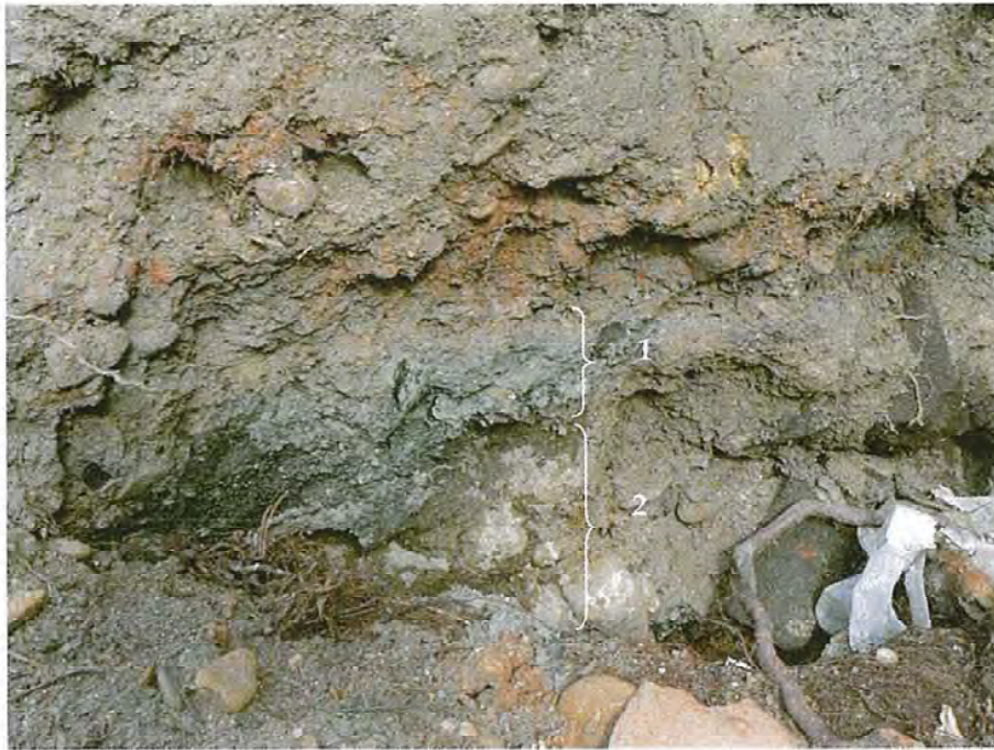
Figure 4.11 Close up of deposits at rear of property showing ash/furnace waste deposit (1) and river gravel (2).
